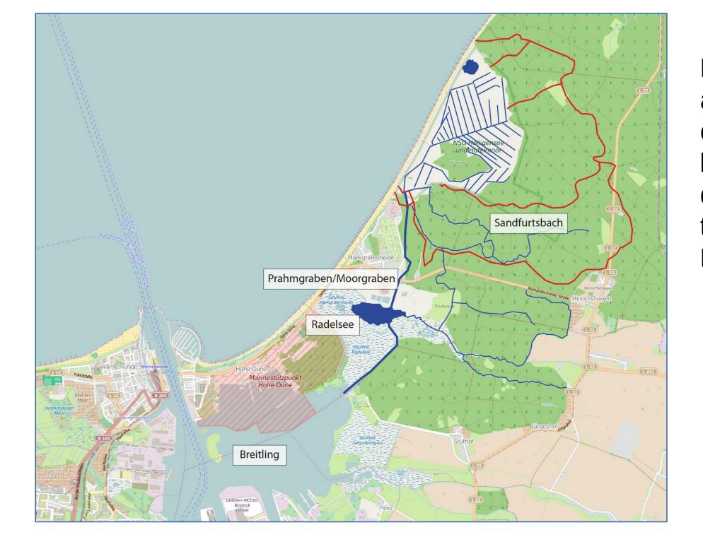
Location of the investigation area (white area at the top right) along the Baltic Sea coast north-eastern of Rostock with the lowland fen, its sub-basins (red lines), its drainage system and its connection with the Breitling via Moorgraben and Radelsee (blue lines) (Miegel et al 2016)
