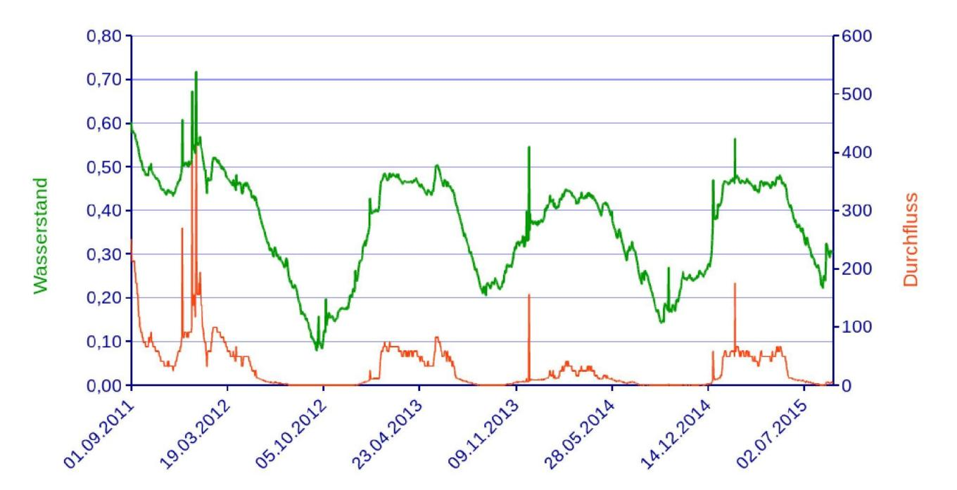
Hydrographs of water level (green line) and discharge (red line) above the groundsill without correction of peaks, caused by backlog events (period September 2011 to August 2015) (Miegel et al. 2016)
